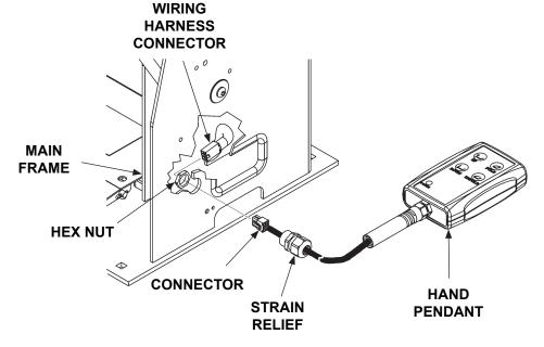
CONNECTING HAND PENDANT CABLE (RH SIDE CONNECTION SHOWN) FIG. 34-1
